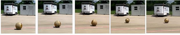
Fig. 8. Screenshots of the shell experiencing a nutation instability, the hubcaps start parallel to the viewer, then shift to perpendicular while maintaining a steady path away
